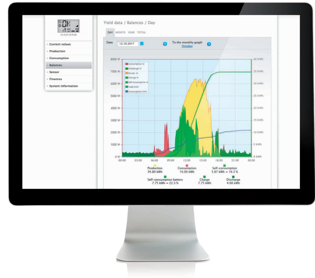
Daily Overview: The battery system is charged when there is a surplus of PV power at the plant (light green) and is used when there is not enough PV power to cover consumption needs, preventing the need to purchase electricity from the grid.
