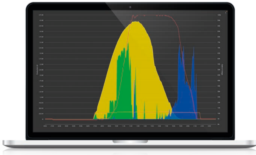
Daily overview: The battery storage is charged with the excess power of the PV system (green) and discharged again if necessary (dark blue) to avoid drawing from the grid.
